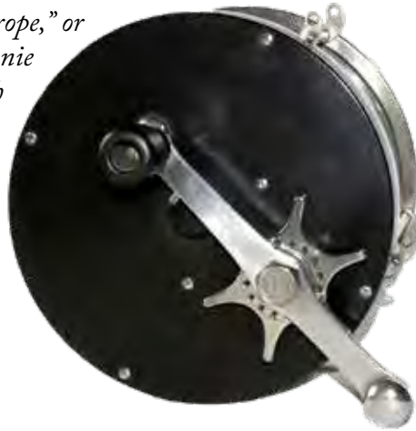
16/0 “Commander” model star drag by Edward von Hoff. E. von Hoff and Joe Cox perfected the star drag reel, a major development in Big Game Reel evolution.
